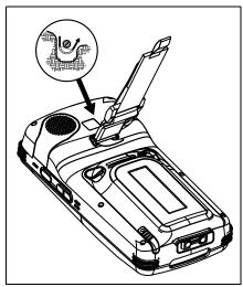
2. Remove the bracket and screws from the Ikôn.
